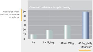
10 µm of coating submitted for an alternated cycling of 8 hours fog cycle (5% NaCl) / dry cycle / humidity cycle. Source: ArcelorMittal Global R&D
