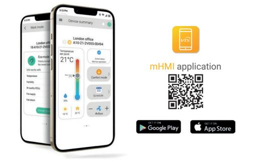
The app connects to the air handling unit using GSM technology (VTS Cloud) or Bluetooth, depending on the user's preference.
